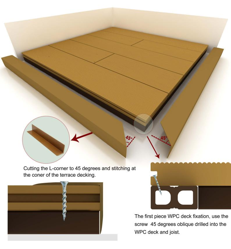
Fixed the L corner with screws to complete the installation.
